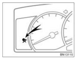
This indicator comes on when the ignition key is turned to the "ON" position. It goes off after about 6 seconds. This means the front seat belt pretensioners are operating properly.
