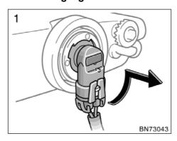
se 2. Pull the bulb out of the base. Install a new bulb.
