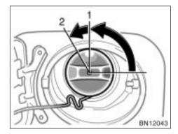
To remove the fuel tank cap, turn the cap counterclockwise by 90 degrees (to the pressure point 1), and then turn it an additional 30 degrees (to point 2). Pause slightly before removing it.
