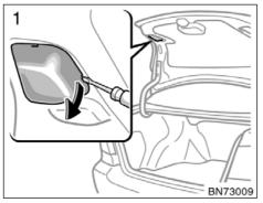
Use a flat-bladed screwdriver or equivalent.
