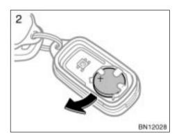
2. Remove the discharged transmitter battery.
