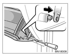
Open the glove box. Remove the screw with a Phillips-head screwdriver and slide off the damper as shown.
