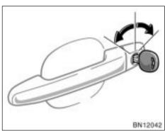
LOCKING AND UNLOCKING WITH KEY Insert the key into the keyhole and turn
