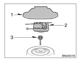
When storing the spare tire, put it in place with the outer side of the wheel facing up. Then secure the tire by repeating the above removal steps in reverse order to prevent it from flying forward during a collision or sudden braking.
