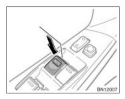
Automatic operation (to open only): Push the switch completely down and then release it. The window will fully open. To stop the window partway, lightly pull the switch up and then release it.
